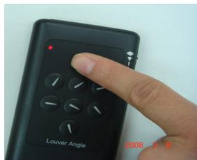
3. To exit from adjustment mode, press the top and the bottom button again at the same time and release, (or don't press any button for 15 seconds). LED light will turn off and remote will resume it standard operational mode.
